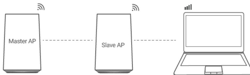
Step1. Place the new AP near the Main Router. Setup connections according to the diagram
