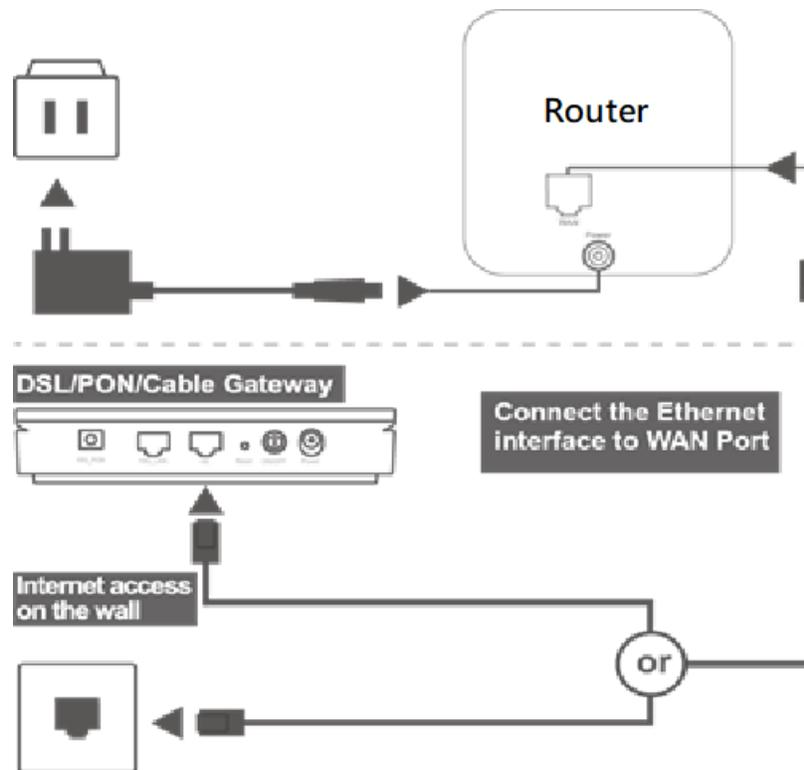
1. Connect the OnBox according to the diagram.
